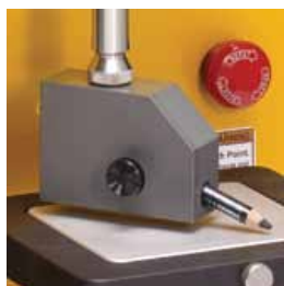
Eye Pencil Fixtures simulates the human force required to apply cosmetic eye pencil as well as the break strength needed to withstand normal applications and packaging/transportation hazards.
