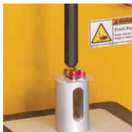
Blister Pack Support accessory imitates the action of a human finger pressing on blister packs to ensure product integrity when extracted from packaging.
