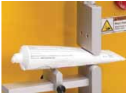
Toothpaste Extrusion Fixture simulates the human force required to test squeezing material out of a tube that comes from the toothpaste industry.
